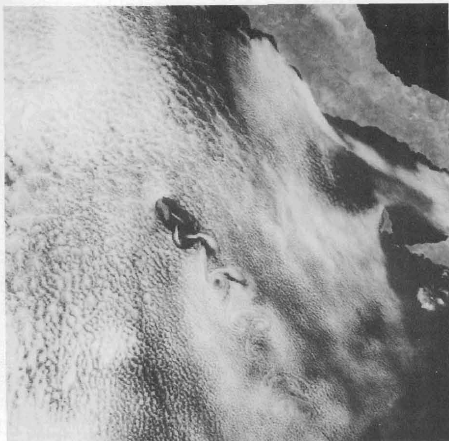
Fig. 1 Photograph of the flow of air past Isla de Guadalupe (Mex.) off the coast of Baja California, obtained at the Atmospheric Environment Service on 25 Aug. 1976 (NOAA 5, Orbit #334). Mist and clouds provide the medium needed to make the flow structure visible.
